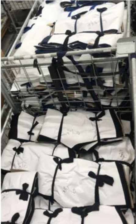
[Re-using cutting scraps as ties for cut pieces]
